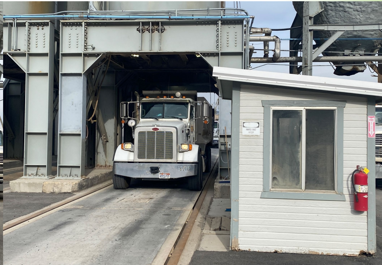
No Smoke – Mix with Chemical WMA at 260F
